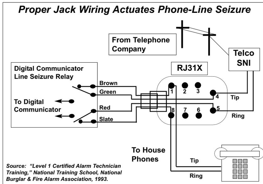
**A properly wired RJ31X jack enables the digital communicator in an alarm control panel to disconnect the telephones inside a premises. This prevents someone from interfering with alarm signal transmission.**
